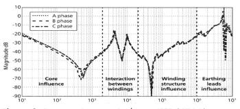
Figure 3: Frequency Response Analysis — IEEE C57.149
