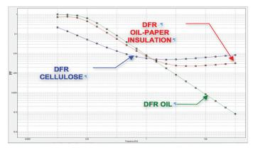
**Figure 5:** DFR of a Transformer's Liquid-Paper Insulation (X=20, Y=20, %mc=1%, s=1E-13 pS/m, T=20°C)
